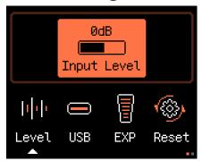
Input Gain: Adjust directly by rotating the VALUE knob, ranging from -20dB to +20dB.
