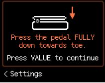
Lower the pedal completely, then press the VALUE knob to confirm.
