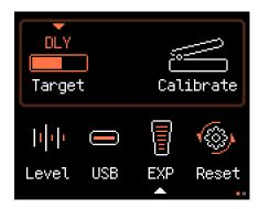
Control Target (Target): Settings for the expression pedal control target, options include None, FX, DRV, AMP, MOD, DLY, RVB.
