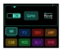
After entering the effect editing of a specific module, rotate the VALUE knob to select a parameter, press to confirm the selected parameter for adjustment. The icon in the upper right corner indicates the current parameter page number; rotating the VALUE knob allows you to turn pages.
