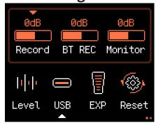
Recording Volume (Record): Volume setting for the USB audio recording effect chain, from -20dB to +20dB. BT Recording Volume (BT REC): Volume setting for USB audio recording of BT audio, from -20dB to +20dB. Monitor Volume (Monitor): Volume setting for USB audio return monitoring, from -20dB to +20dB.
