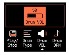
Rotate the VALUE knob to change the drum machine playback volume.
