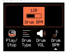
Rotate the VALUE knob to change the drum machine playback speed.
