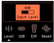
In the global settings interface, press the GLOBAL button to switch between settings, with the page number displayed in the lower right corner.
